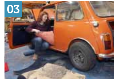
After removing the securing screws for the gear lever gaiter and undoing the bolts for the seatbelt stalks, we can remove the one-piece carpet and any underlay and old soundproofing material. Luckily, everything on the floor area is dry.
