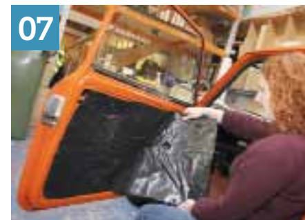
Sophie suspects water is getting past the door seals and the weatherstrips. The plastic waterproof sheeting on the doors is wet. Inside the doors, the drain holes are clear and the metalwork is dry.
