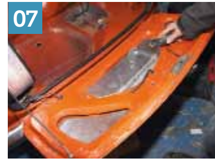
The inside of the boot panel can be lined where the outer skin is exposed. This panel vibrates when we tap it so three pre-cut pieces of barrier mat are stuck to it to reduce noise amplification.
