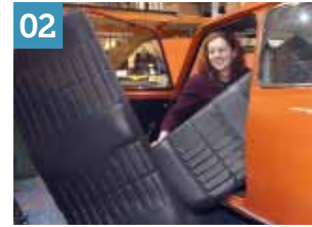
The base of the back seat isn't secured in position so it can be pulled free and removed. The seat back is clipped at the top to the rear bulkhead. We'll be fitting self-adhesive barrier mat to the bulkhead and barrier mat underneath the seat base.
