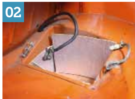
Tapping the sides of the battery box reveals lots of unwanted vibrations and noise, which can be deadened with self-adhesive barrier mat. We decide to cover the sides of the battery box but not the floor because water occasionally collects here.
