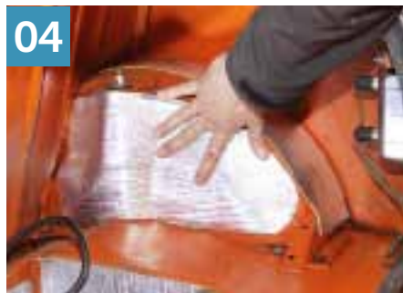
The wheel arches transmit and amplify lots of road noise from the tyres, so these should be covered wherever possible, on the inside of the Mini, with barrier mat. We start on the offside rear (OSR) wheel arch in the boot.
