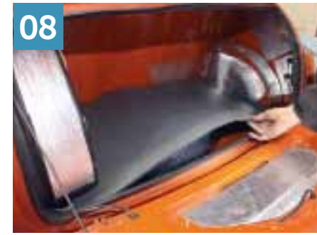
The inside of the boot panel can be lined where the outer skin is exposed. This panel vibrates when we tap it so three pre-cut pieces of barrier mat are stuck to it to reduce noise amplification.
