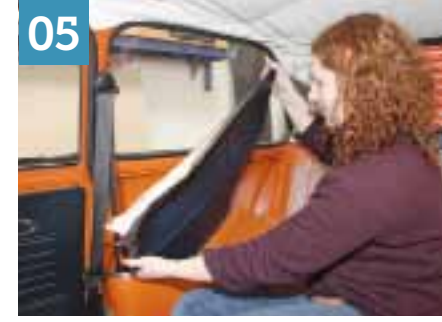
The rear side trim panels hide a vast area of metal that vibrates and amplifies sound, particularly from the tyres, so we remove them, along with anything that covers the rear wheel arches, as these will also be soundproofed.
