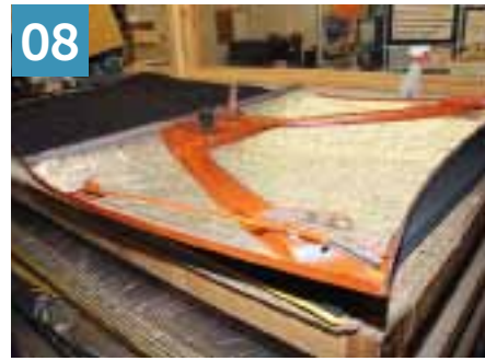
The underside of the bonnet is now fully covered in Vibrasorb (except for the framework) and a decorator's roller is used firmly to stick the material to the metalwork. This will help to absorb engine noise and reduce panel vibration.
