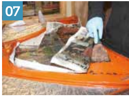
With the bonnet laid on a flat surface, Grant Bithell at Noisekiller scrapes off the remaining brittle, old soundproofing material, then uses newspaper soaked in white spirit to remove any adhesive that has been left behind.
