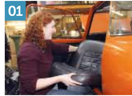
It isn't always necessary to remove the seats and carpets to fit sound deadening material, as it can be squeezed underneath the carpets, but we decide to strip the interior, starting with the front seats, which are secured with 3/8-inch bolts.
