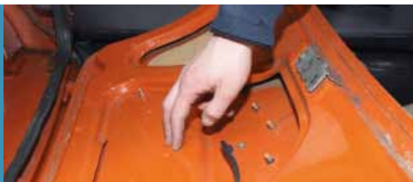
The inside of the OSR quarter panel vibrates when we tap it with our fingers, so it needs to be covered with barrier mat. There's room to fit three pre-cut pieces, then firmly stick them to the metal using a roller.
