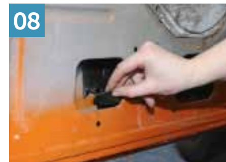
Sophie suspects water is getting past the door seals and the weatherstrips. The plastic waterproof sheeting on the doors is wet. Inside the doors, the drain holes are clear and the metalwork is dry.
