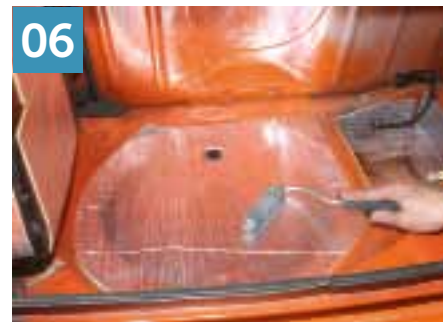
The spare wheel well amplifies noise from the exhaust silencer, so we fit a large piece of barrier mat, but cut out a square for the drain hole, which is plugged with a rubber grommet (water can collect here).
