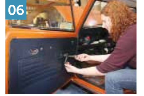
We're intending to soundproof inside the doors, so remove the door cards. These are secured with screws for the window winder handle, release and pull handles, plus several plastic clips, some of which break when we remove the card.
