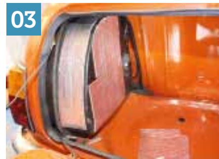
The petrol tank is effectively a large drum, which amplifies lots of sound, so three pieces of barrier mat are stuck to the edge and side. If required, we could remove the tank and cover all of it with the material, but this should be sufficient.
