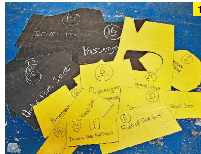
Above left: it might look like a giant jigsaw but, fortunately, all the pre-cut soundproofing sections have their positions marked for easy fitting.
