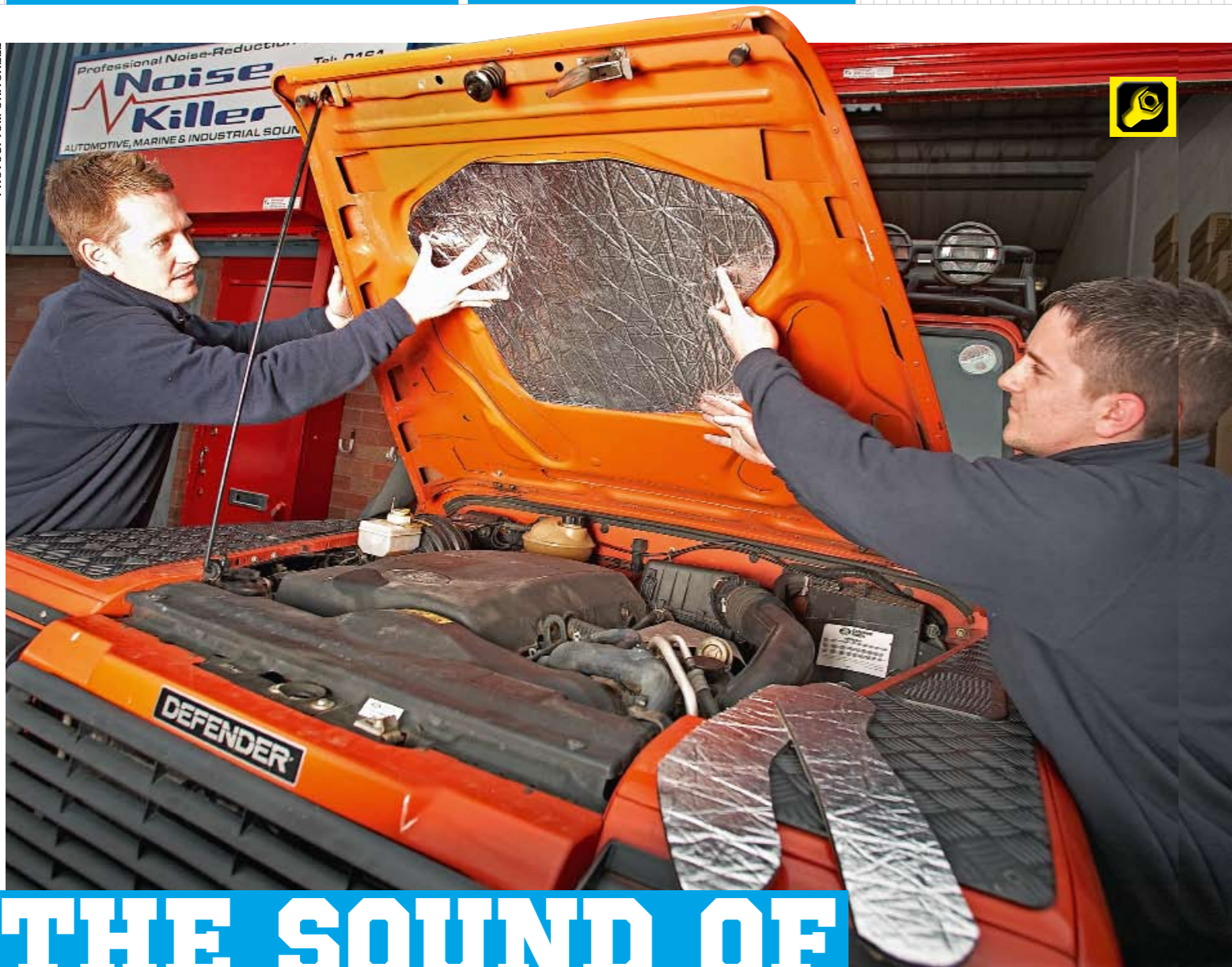
Above left: it might look like a giant jigsaw but, fortunately, all the pre-cut soundproofing sections have their positions marked for easy fitting.
