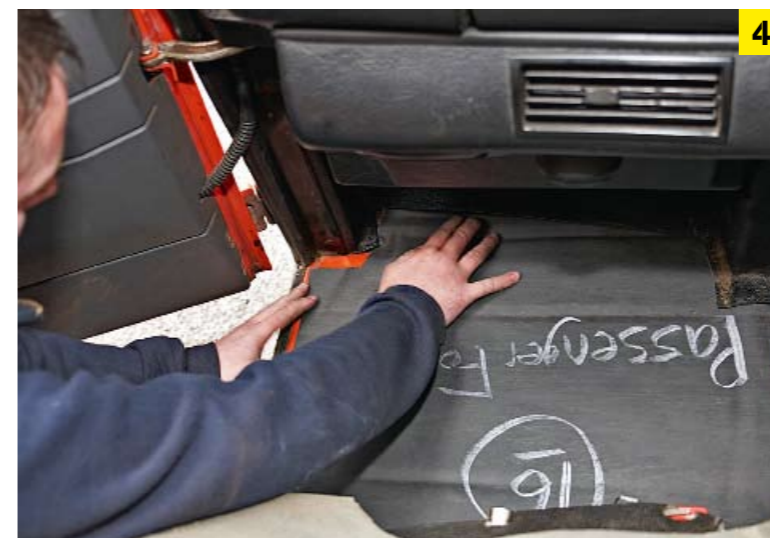
You have to wrestle out the front mat or carpet before fitting the two footwell sections. The aircon on my vehicle prevents another section being fitted to the bulkhead, and this side panel has to be cut around the aircon pipe. The driver's side is worse because you have to fit it around the pedals and handbrake.
