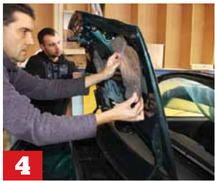
4 Trial fit each piece of Vibrasorb to the underside of the boot lid. It may be a tight fit around the edges, so trim it if necessary. When you're ready, peel off the backing paper and secure each piece in position.
