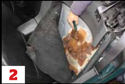
2 Make sure the metal panel of the firewall is clean. If necessary, scrape off any rust or old soundproofing. Two pieces of self-adhesive barrier mat need to be stuck to this surface, so remove any loose dirt and rust.
