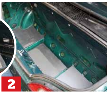
2 Three pieces of pre-cut sound barrier can be fitted on the boot floor. These will help to absorb noise from the exhaust, which is amplified inside the boot. Make sure the boot floor is dry before fitting them.
