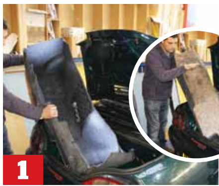
1 Carefully prise out all the plastic plugs that secure the moulded carpet inside the boot. Manoeuvre the carpet out of the boot and check the condition of the soundproofing material on the underside. If it is soggy, either remove it or dry it out.
