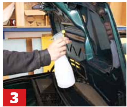
3 Two pieces of Vibrasorb can be fitted to the underside of the boot lid. First, spray over the surfaces to be covered with panel wipe to remove any dirt and oil - this area can get contaminated with oil from the engine.
