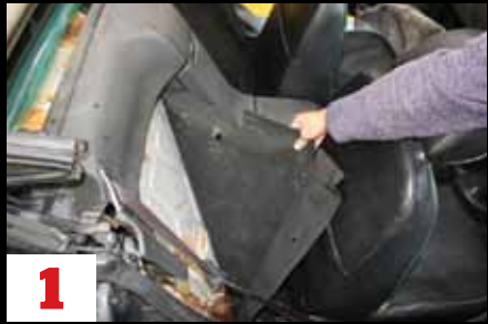
1 Unscrew the plastic fittings that secure the carpet over the rear firewall. Peel back the carpeting - it cannot be fully removed as it's fitted behind the centre console. Remove any old soundproofing material from behind it.
