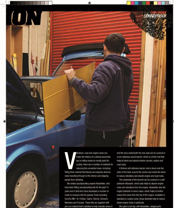
We spent a full day with Noisekiller, stripping the interior of Ben Clapinson's Mk4 Escort and fitting the aforementioned soundproofing material. He was amazed by the difference the soundproofing has made. The following pages outline the work involved.
