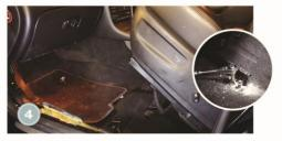
After removing the plastic cover, we can now see the last two 10mm bolts and undo them. The seat is now loose, but we do not remove it otherwise we would need to first detach its electrics.
