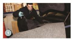
.The spare wheel and the carpet over it are easily removed. Next, use a selection of plastic trim tools to release some locating plugs to allow you to remove the remaining trim and carpeting.
