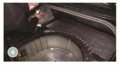
The pre-cut pieces of adhesive barrier mat are trial-fitted inside the boot to check they are the correct size. After peeling off the backing paper stick them in position and press down firmly using a decorator's roller.
