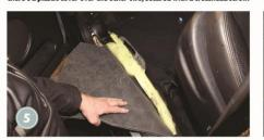
Instead, with the seat tilted into the rear footwell, there's room to squeeze a thick, pre-cut piece of sound barrier under the front carpet and into the front footwell. Space is tight and the carpet is strong.
