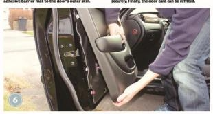
The front door cards are secured by the same means as the rear doors, with two screws along the bottom and one in the centre (hidden by a cover). The waterproof foam needs to be carefully peeled off to get inside the door.
