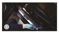
We're going to fit sound barrier underneath the carpets, but want to see if this can be done without fully removing the seats and detaching any electrics. First, we remove the plastic trim and the sills.
