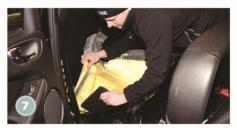
The front seat is moved forwards and there's room to slide another pre-cut piece of sound barrier under the carpet and into the rear footwell. The pieces of sound barrier are smaller than the front pieces and there's lots of room.
