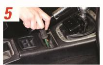
The centre console needs to be removed if you want to soundproof the propshaft tunnel. Remove the box inside the ashtray, then undo two crosshead screws. Undo more crosshead screws inside the lockable companyment.
