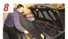
The final piece of soundproofing for the boot consists of a large sheet of non-adhesive sound barrier. This can be fitted under the boot carpet and helps to reduce vibrations and block road and exhaust noise.
