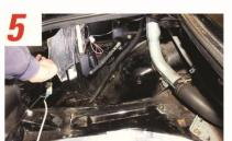
Small pieces of self-adhesive barrier mat can be fitted inside the rear wings. There's not much room to fit these. Tap the panels to see where the noise is generated, then trial fit a piece or two in position.
