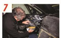
Peel back the plastic waterproof sheeting to see where the barrier mat can be fitted inside the door. Use small pieces and see if they can be easily fed into position without sticking to everything.
