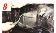
After fitting a few pieces of self-adhesive barrier mat, make sure they are securely stuck down by running over them with a decorator's roller. Water will drip down the inside of the door, so the barrier mat must be secure.
