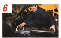
Prise up the switch panel for the electric windows and disconnect the plug. Undo the retaining screws at the side of the centre console. Unscrew the gear knob and you should now be able to lift off the centre
